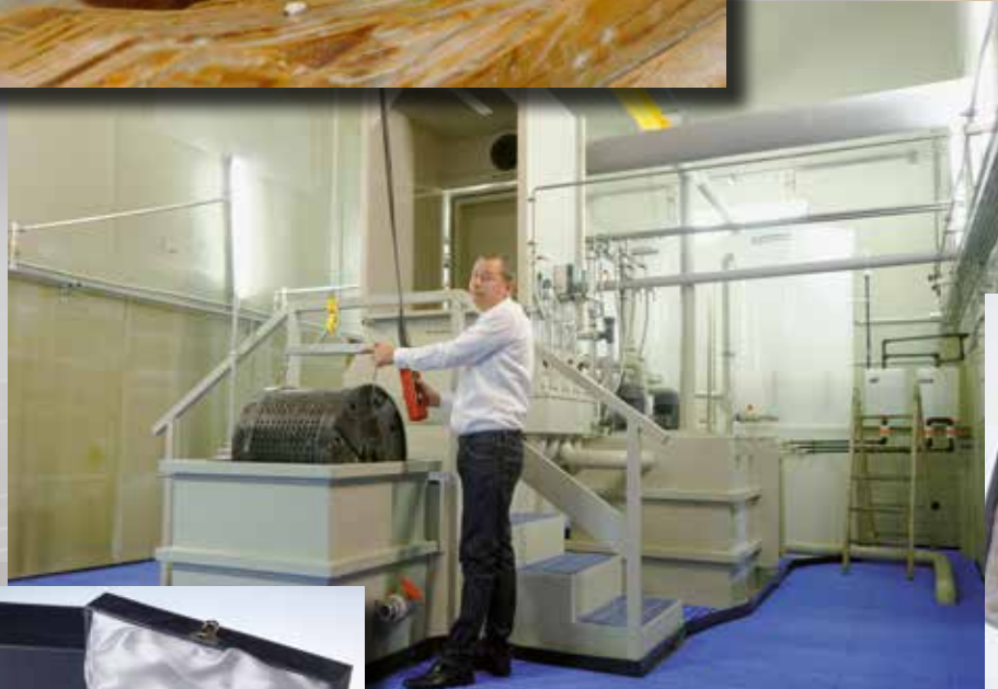
ACIDIC POLISHING ACIDIC POLISHING GIVES CUT OBJECTS A SPARKLING, SHINY FINISH BY DIPPING THEM IN A MIXTURE OF HYDROCHLORIC AND SULFURIC ACID FOR ABOUT 35 MINUTES. IT IS ESSENTIAL TO PROPERLY CONTROL THIS UNSTABLE MIXTURE AS A VARIATION OF 2% TO 3% WILL MAKE ALL THE DIFFERENCE TO THE QUALITY OF THE FINAL PRODUCT.
