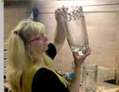
CHECKING OF GLASSES AFTER POLISHING
